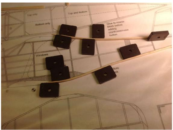
a. Soak the wood, stack the pieces and shape to match the curves of the fuselage. This will make for a stronger fuselage and less prone to breaking.
