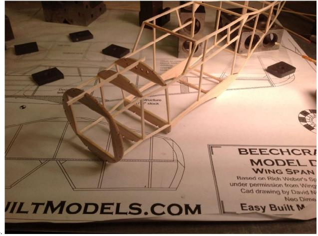
a. Start adding the stringers around the nose. I like to work symmetrically, put on the top stringer then the bottom, one center side piece then the opposite always paying attention to keeping everything straight and the fuselage sides aligned. It takes effort but you can make your fuselage straight and symmetrical with care and this goes a long way towards having a great flying model.
