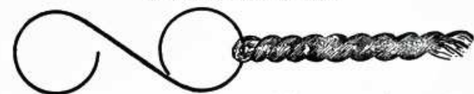
Fig. 2.—Stranded rubber motors should be connected to a strong S-shaped hook, as here, the open end of the hook then being coupled to the propeller shaft.
