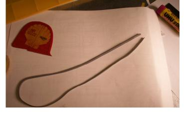
You start by laying out the rubber in a single loop, you can then twist it halfway down the loop and double it over creating a double loop half the length with twice the power.
