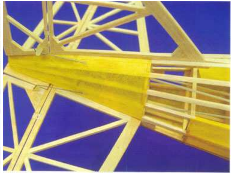
For the threading of the control rods, balsa is set into the spaces between the stringers.
