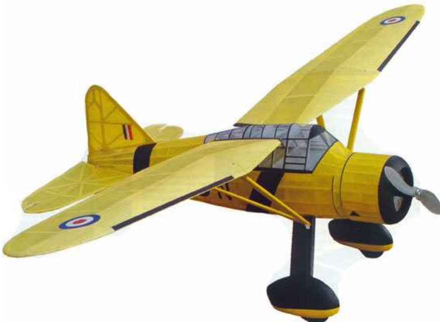
The Lysander is clad with 12 g paper in the colours of a target drag machine. The emblems and insignia too, are made of paper.
