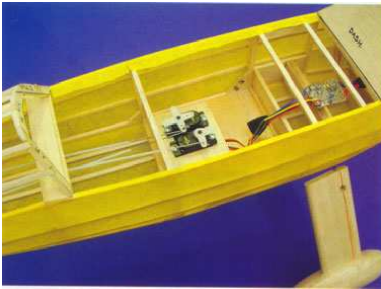
In the large fuselage, there is ample room for the receiver and servos
