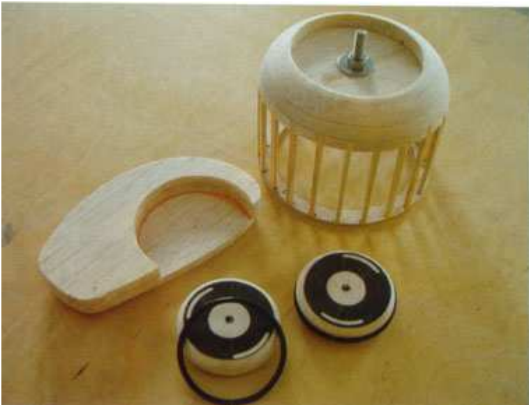
The wheels with notch and O – ring and a half completed spat. Next to it, the sanded motor cowling.
