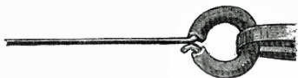
Fig. 1.—A cycle valve-tube slipped over the hooks carrying the rubber motor will double the life of the elastic by preventing cut strands.
