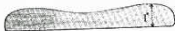
Fig. 12. The propeller, cut from a piece of birch, as it appears before being twisted.
