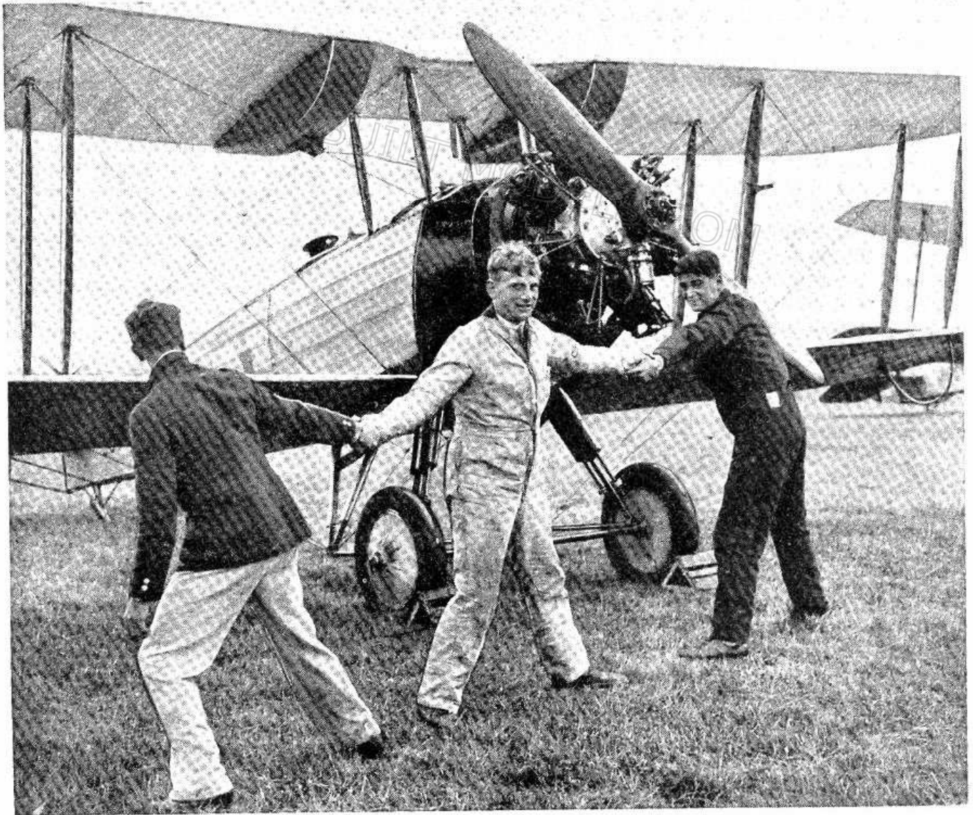
Starting up an aeroplane's engine by swinging the propeller is not so easy as it looks !
