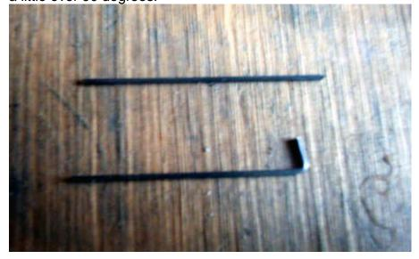
Cut a section of 0.185 I.D. x 0.25 O.D. steel tubing a little over 3/8" long for the hub. Grind ends parallel to 3/8 final length. (This will wind up accommodating an axle 0.110" in diameter or smaller. To use a larger axle, use a larger inside diameter tube.)
