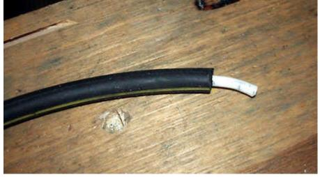
Clamp a 2" PVC union in a vise. Wipe the inside with a rag and a tiny amount of light oil to serve as a release. Mix fast setting epoxy, coat the insides of the hose ends for at least ½", coat the insert, put it in the hose and join the ends, making sure the insert bridges the gap. Press the tire into the bore of the PVC, align the joint and wipe off the excess epoxy.
