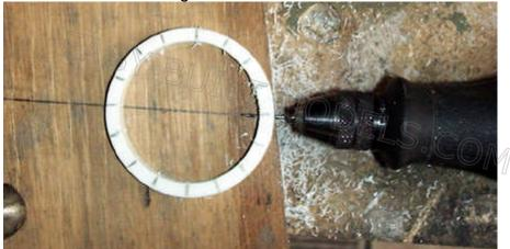
Bevel the inside diameter and round the edge of the outside diameter of the rim.
