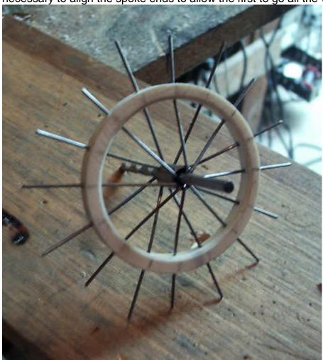
Make sure all spokes are pulled out so that the bent ends are in contact with the hub and properly positioned. Trim the spokes with cutters. Put a shallow 0.110" hole in the center of the circle used to layout the spokes. Rest the end of the inserted drill in the hole and turn the wheel, checking for runout against the circle on the board. Holding the hub with the drill, push the rim in the proper direction to get the hub reasonably centered.
