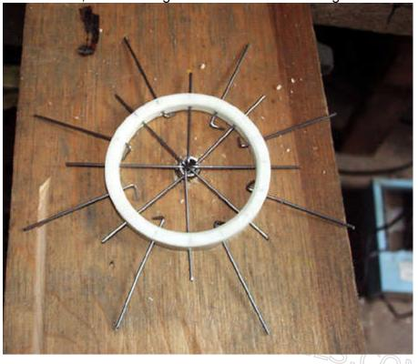
Slide a 0.110" (#35) drill bit through the hub (a second one started from the opposite side may be necessary to align the spoke ends to allow the first to go all the way through.)
