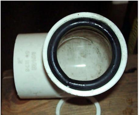
Allow the epoxy to set to full strength. Remove the tire and sand or file the joint smooth. If there are gaps, they can be filled with black aquarium sealer or any other black rubber filler or adhesive.
