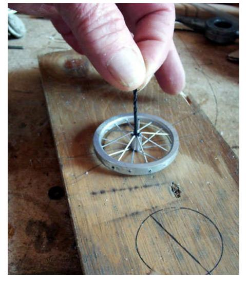
Place the wheel horizontally on a flat surface and press the hub down. Visually verify that the rim is the same height off the surface all the way around. If not, gently push the high spot down. Recheck the wheel for roundness.
