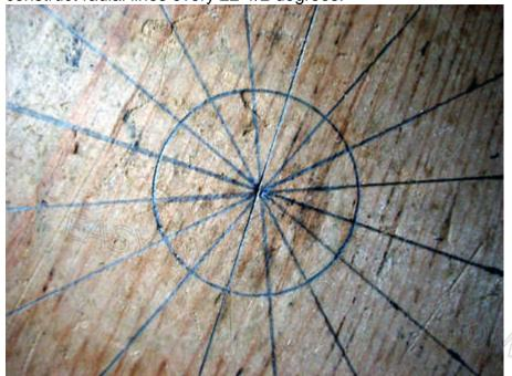
Place the rim over the circle and mark the perimeter in line with the 22-1/2 degree marks.
