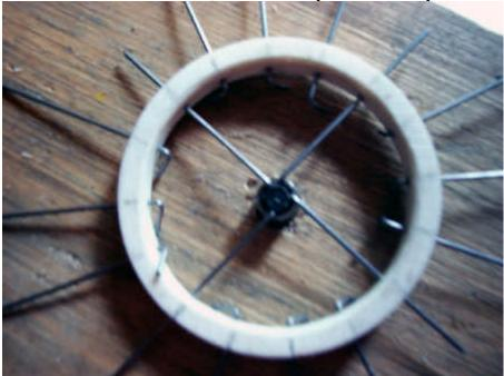
Install the other 2 at 90 degrees to the first 2 on this side, then 2 more across from each other at the 45 degree points on this side. Turn over, remove the hub filler material and install the remaining 4 on the first side, then over again to install the remaining 2 on the other side.
