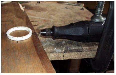
Carefully slide the rim into the bit at each marked location to drill 16 spoke holes. Keep the rim square with the bit when drilling.
