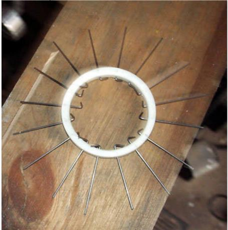
Drill a 9/32" diameter hole in a board about 1/8" deep. Set the hub in the hole and set the rim over it. Using needle-nose pliers, hook 4 spokes spaced 90 degrees apart over the hub. (Note that the 8 spokes on one side are all one mark (22-1/2 degrees) from those installed on the opposite side.
