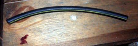
Cut a 1-1/2" length of round plastic that fits snugly into the hose. (Jacketed 4-conductor 22 gage
