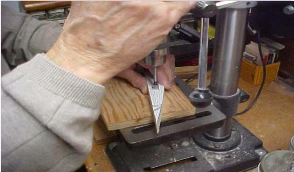
**These particular ribs have a square hole that needs to be made through all ten ribs. Choose a fosner bit and center it in the intended hole. Chose a bit that is close to the sides to remove as much material as possible, making a round hole into a square hole. I prefer this to using a scroll saw. Scroll saws want to wander from side to side and you cannot get a clean square cut. By removing as much material as possible another tool that you can make yourself makes a better square hole.**
