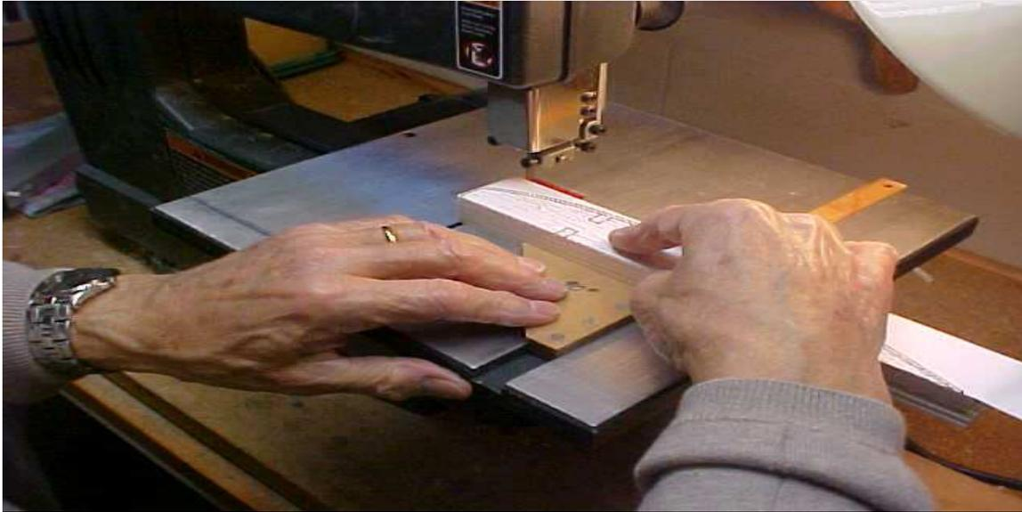
**I use a square with my band saw to cut the front of the rib to 90 degrees or what ever is required. The band saw cut straight unlike a scroll saw. Use a metal cutting blade as it has more teeth and a smother cut is made in the soft balsa.**
