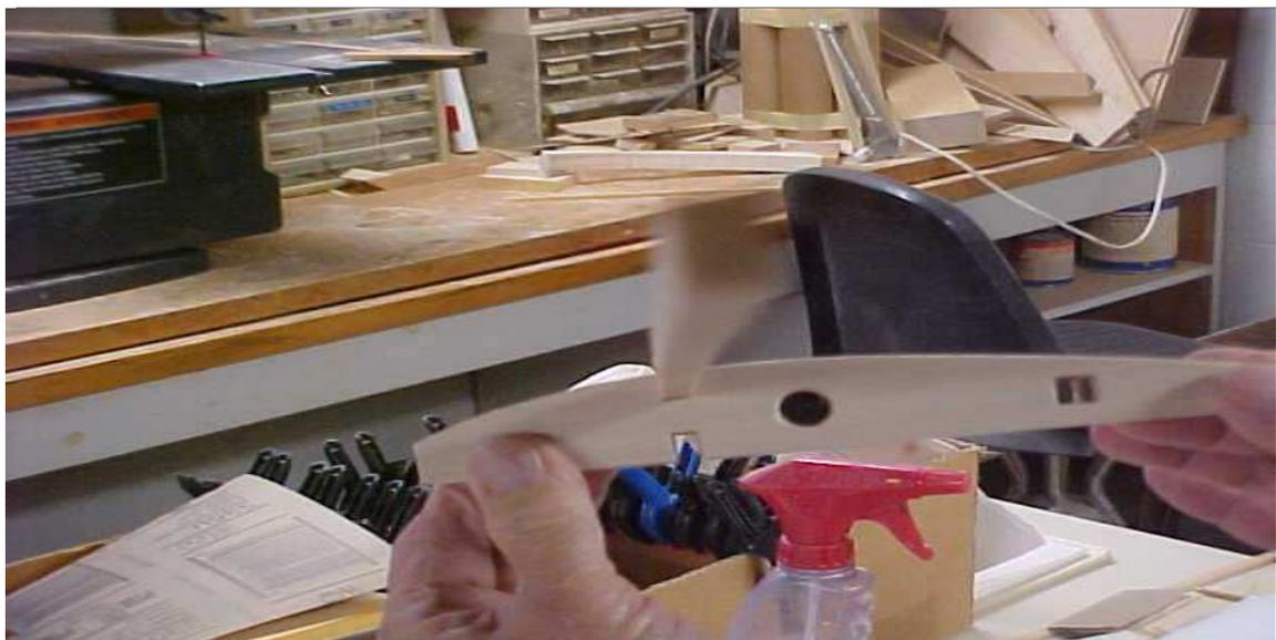
**Spar is test fitted through all ten ribs top bottom. Note round hole which will be used for the wiring of the servo. Note the square hole. That was also test fitted with the spar for proper fit.**
