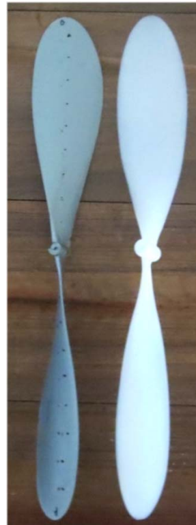
Fig. 1. Peck (gray) and EBM (white) 9.5" propellers.
